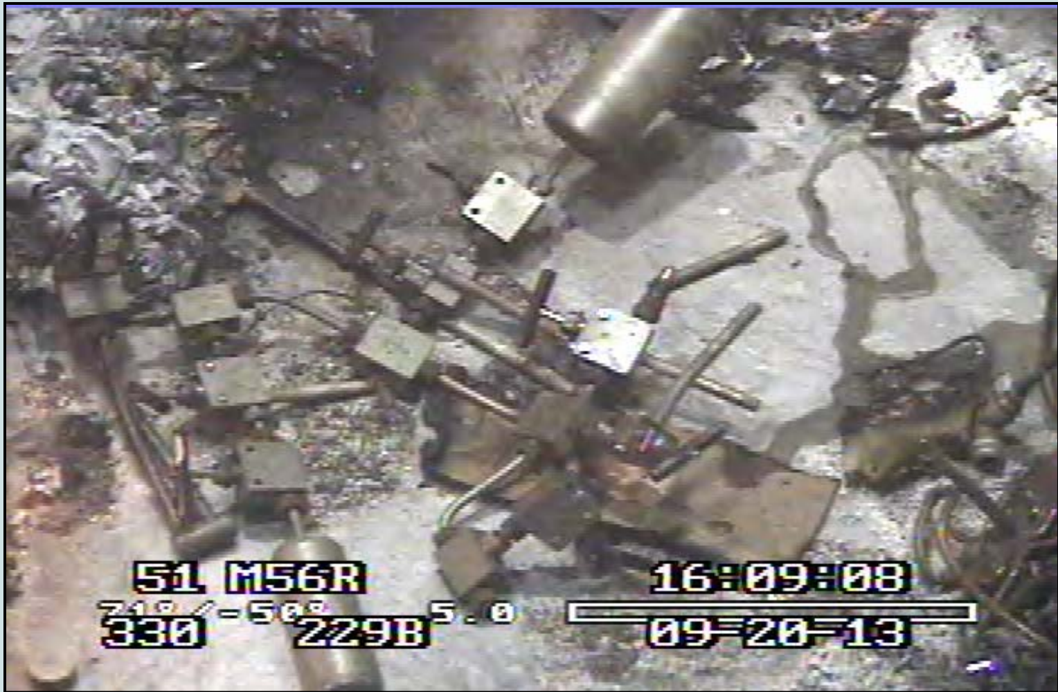
View of North Box Line processing trough after fire event.
